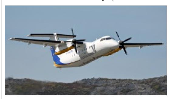
The standard MTOW of 36,300 lbs is increased to 37,300 lbs for three aircraft operational configurations:
